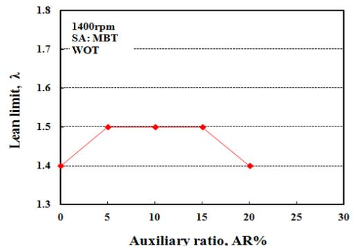
Fig. 4 Lean limit as a function of auxiliary ratio, AR(%)
