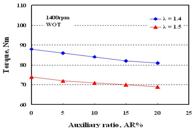
Fig. 6 Torque as a function of auxiliary ratio, AR (%)
