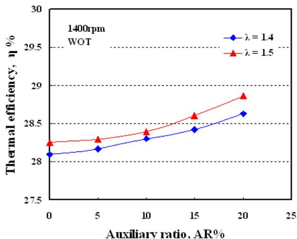
Fig. 5 Thermal efficiency as function of auxiliary ratio, AR (%)
