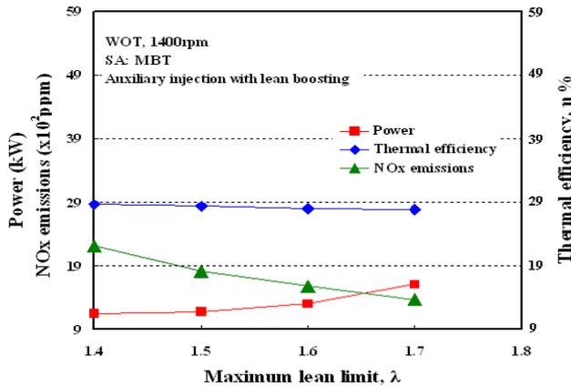
Fig. 8 NOx emissions, thermal efficiency and power as function of maximum lean limit, ( $\lambda$ )
