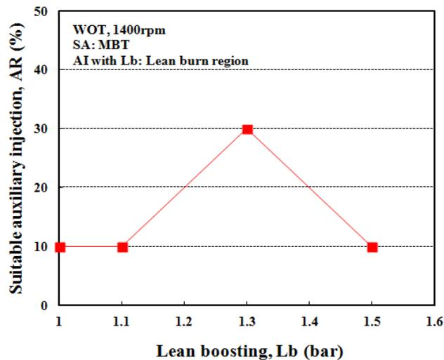
Fig. 9 Auxiliary injection ratio required to lean boosting
