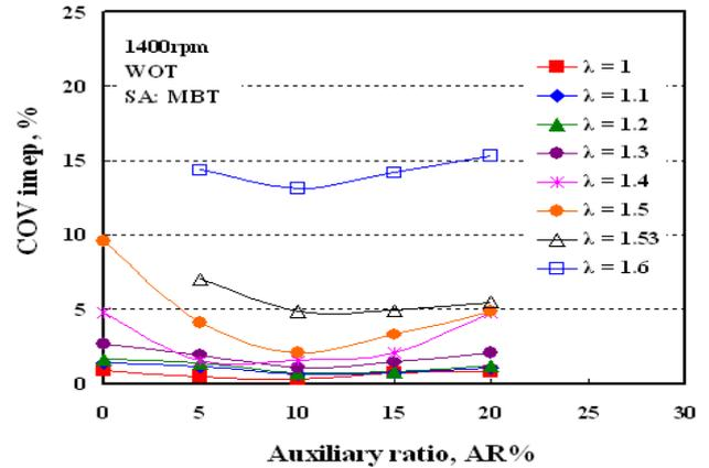
Fig. 3 COV imep as a function of auxiliary ratio, AR(%)
