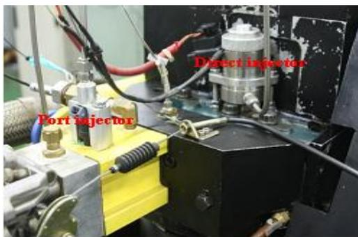
Fig. 2 Location of port and direct injectors
