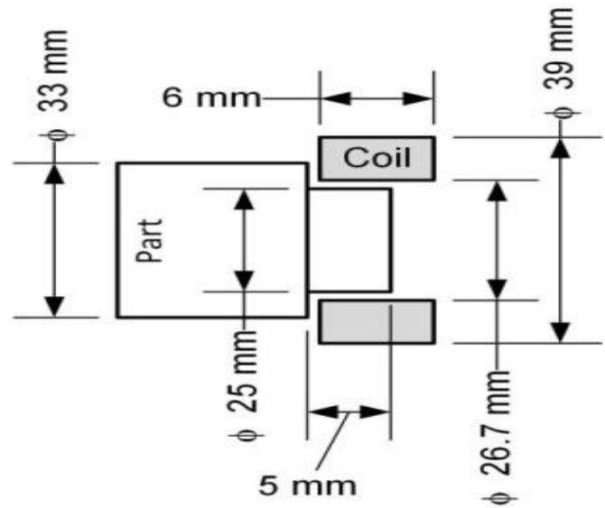
Fig. 1. Bearing seating and coil dimensions
