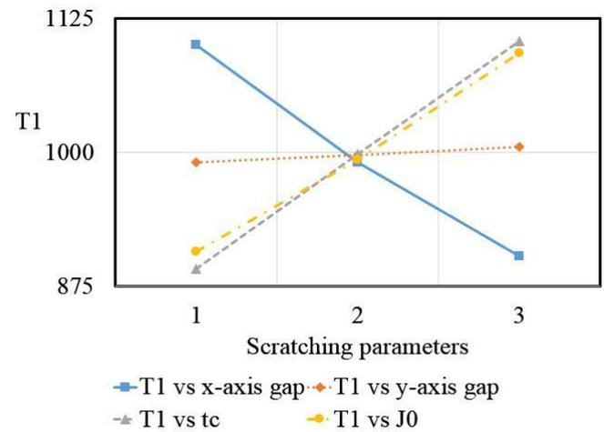
Fig. 10. Main effects of x-axis gap, y-axis gap,  $\tau$ , and  $J_0$  on T1(°C).
