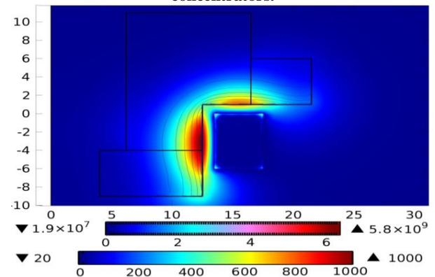
Fig. 5. Temperature distribution (°C) [0,1000] and total induced current ( A · m) [1.9x 10<sup>7</sup>, 5.8x 10<sup>9</sup> ] using flux concentrators.
