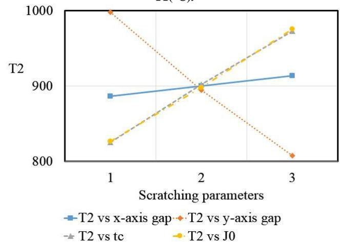
Fig. 11. Main effects of x-axis gap, y-axis gap,  $\tau$ , and  $J_0$  on T2(°C).
