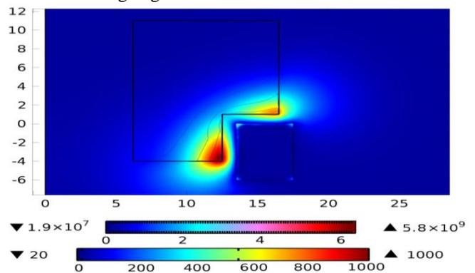
Fig. 4. Temperature distribution (°C) [0,1000] and total induced current ( A · m) [1.9x 10<sup>7</sup>, 5.8x 10<sup>9</sup> ] without flux concentrators.
