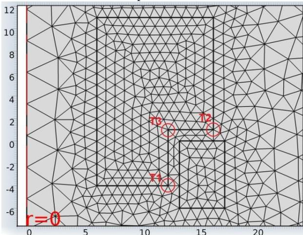
Fig. 2. Space discretization (mesh) in COMSOL
