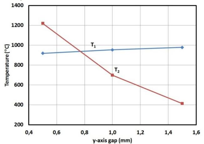
Fig. 7. T1 and T2 versus y-axis gap.
