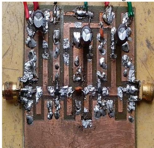
Fig 9: The fabricated LNA
