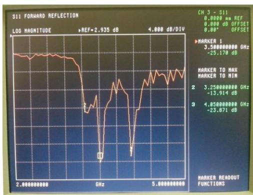
Fig 11: The input reflection coefficient  $S_{11}$
