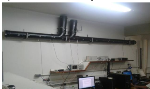
Fig.3: Duct experimental built at the Laboratory of Acoustics and Vibration UFU.
