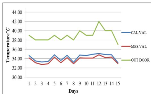
Fig.5 Comparison of measured and calculated indoor temperature and outdoor temperature
