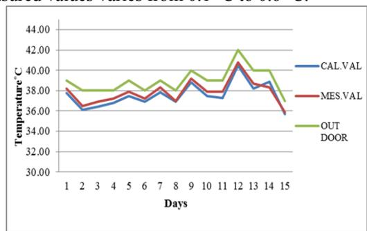
Fig – 4 comparison of the indoor ambient measured and calculated
