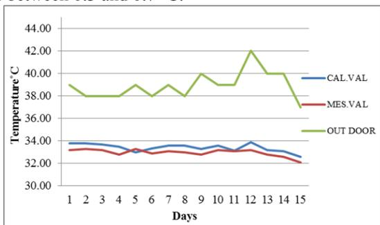
Fig.6 Comparison of measured and calculated indoor temperature and outdoor temperature
