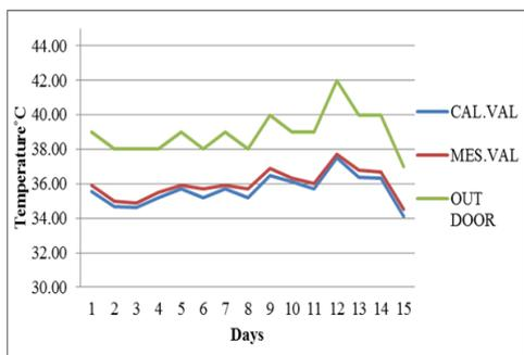
Fig.7 Comparison of measured and calculated indoor temperature and outdoor temperature
