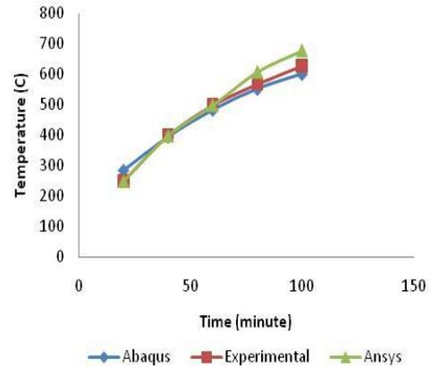
Fig 4. Comparison of Temperature at the Reinforcement Performed by Ansys, Abaqus 3D Model and Experimental Test.
