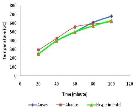
**Fig 9. Comparison of Temperature at the Reinforcement Performed by Ansys, Abaqus 2D Model and Experimental Test.**
