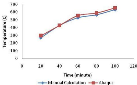
**Fig 8. Comparison of Temperature at the Reinforcement Performed Abaqus 2D Model and Manual Calculation**
