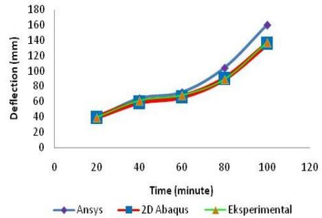
**Fig 10. Shows the maximum deflection result at the mid span of the slab performed by Abaqus**
