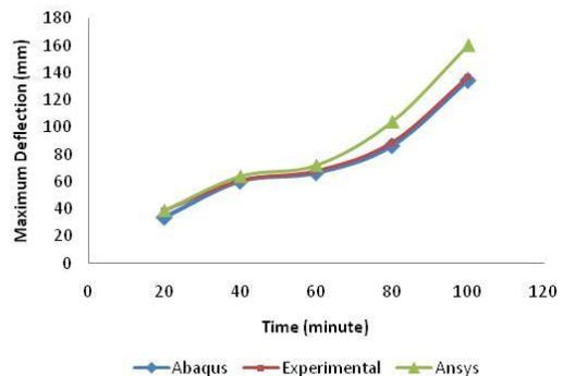
Fig 5 Comparison of Maximum Deflection at Mid Span of Slab Performed by Abaqus, Ansys and Experimental Test.
