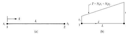
**Fig 1. Basic One dimensional temperature element (b) Temperature Variation along the Length of the Element**
