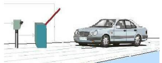
Fig 3: step three: The vehicle is allowed to enter if it is authorized.
