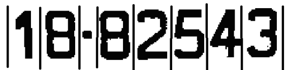
Fig 15: Segmentation by projection
