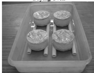
Fig.3. Concrete Specimens during Sorptivity Test
