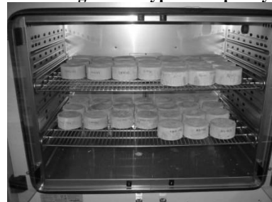
Fig.2. Pre-Conditioning of Sorptivity Specimens inside the Drying Oven
