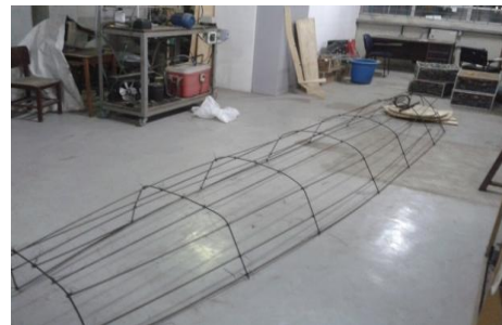
Fig 8 – Frame of the hull
