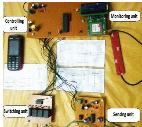
Fig: 8 Implementation of final hardware circuit design
