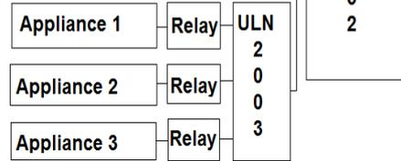
Fig: 7 Block Diagram of Switching Unit
