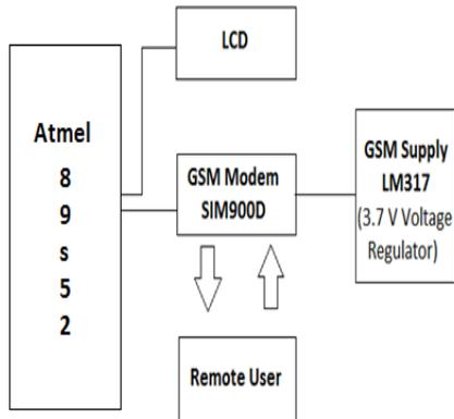
Fig: 6 Block Diagram of monitoring unit
