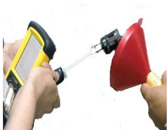
Picture 1. Taking physico- chemical sample of the medical air.
