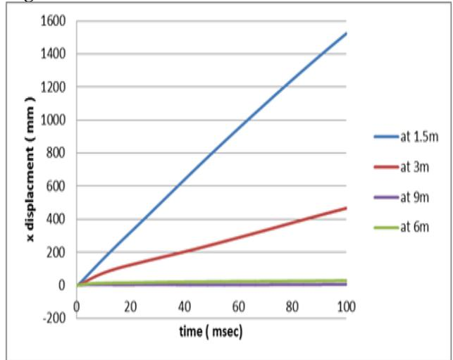
Fig.15: x-displacement histories of at mid height of column C2 of building B – load case 1.
