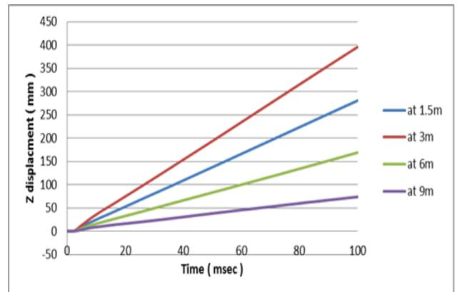
Fig.12: z-displacement histories of at mid height of column C3 of building A – load case 2.
