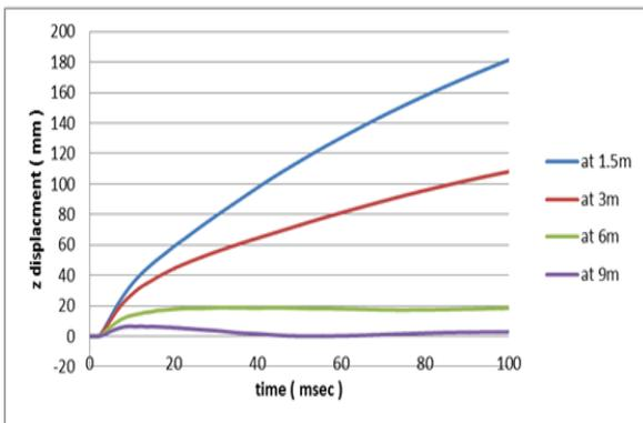
Fig.18: z-displacement histories of at mid height of column C2 of building B – load case 2.
