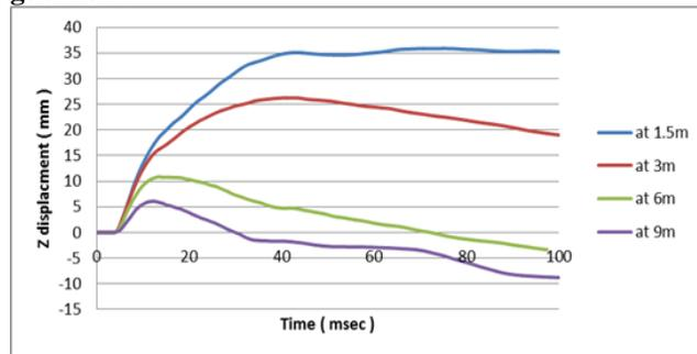
**Fig.24: z-displacement histories of at mid height of column C2 of building C – load case 2.**
