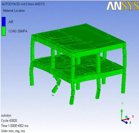
Fig.13: deformed shape of building B due to blast load at 1.5m from the middle column.
