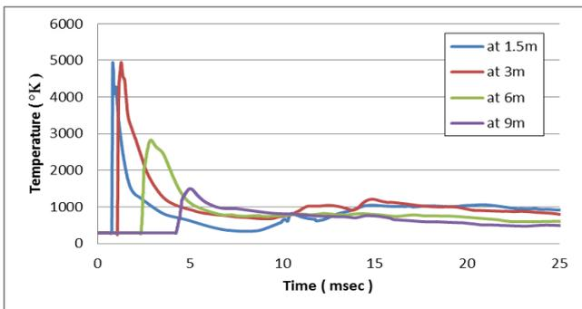
**Fig.6:** temperature histories at mid height of column C1 of building A - load case 1.
