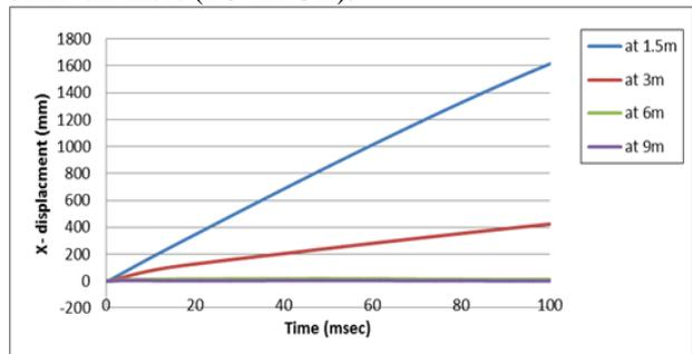
Fig.21: x-displacement histories of at mid height of column C2 of building C – load case 1.
