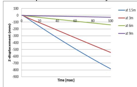
**Fig.7:** z-displacement histories of at mid height of column C1 of building A – load case 1.
