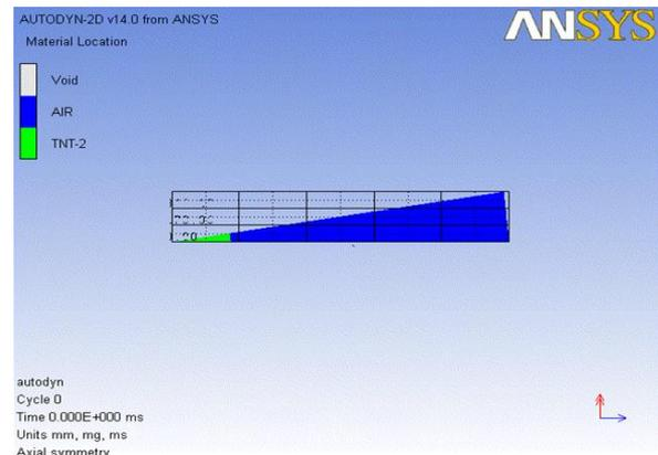
Fig.2: 1D wedge filled with TNT and air modeled with multi material Eulerian formulation.
