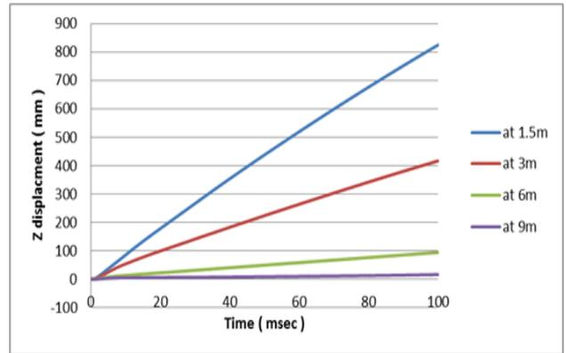
Fig.11: z-displacement histories of at mid height of column C2 of building A – load case 2.
