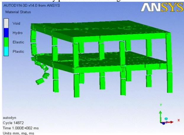
**Fig.22:deformed shape of building C due to blast load at 1.5m from the corner column.**
