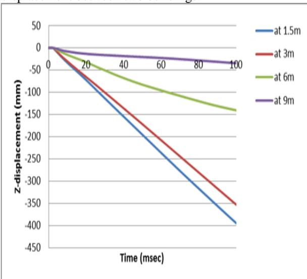
Fig.14: z-displacement histories of at mid height of column C1 of building B – load case 1.
