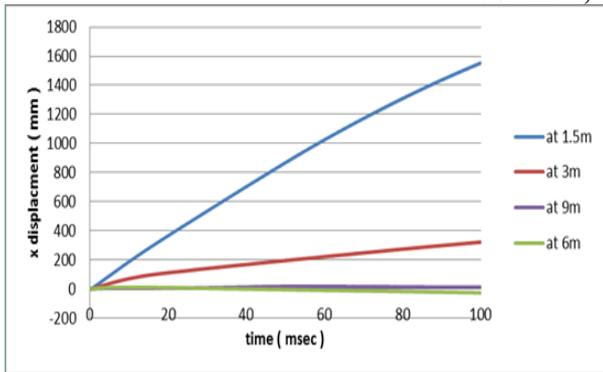
Fig.17: x-displacement histories of at mid height of column C1 of building B – load case 2.
