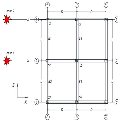
**Fig. 3 Plan of the building and Location of Blast.**
