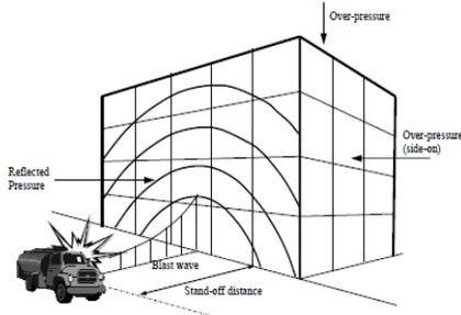
Fig.1: blast loads on a building [13]
