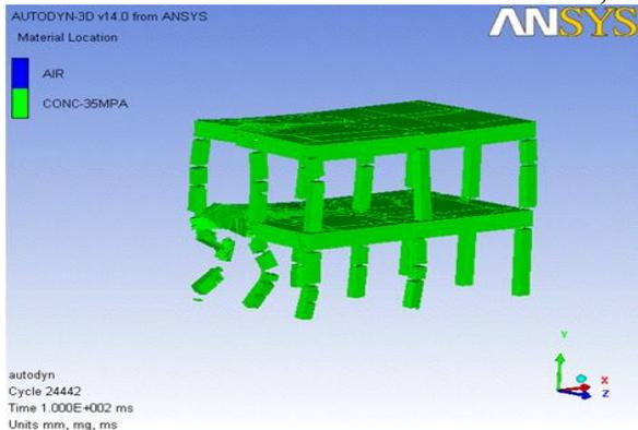
Fig.9: deformed shape of building A due to blast load at 1.5m from the corner column.
