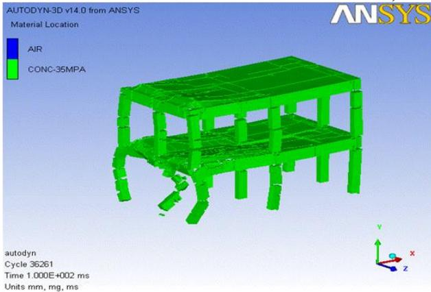
**Fig.4:** deformed shape of building A due to blast load at 1.5m from the middle column.
