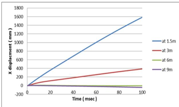
Fig.10: x-displacement histories of at mid height of column C1 of building A – load case 2.
