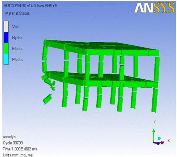
Fig.16: deformed shape of building B due to blast load at 1.5m from the corner column.
