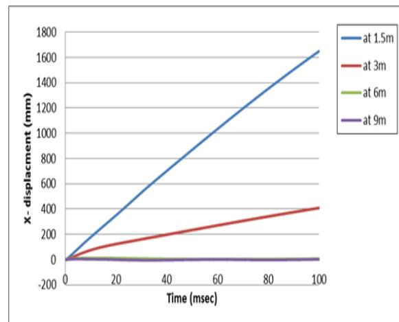
**Fig.8:** x-displacement histories of at mid height of column C2 of building A - load case 1.
