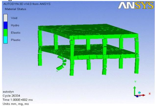
Fig.19: deformed shape of building C due to blast load at 1.5m from the middle column.
