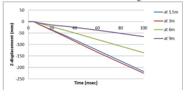
Fig.20: z-displacement histories of at mid height of column C1 of building C – load case 1.
