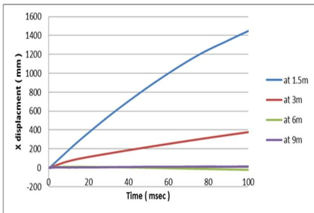
**Fig.23: x-displacement histories of at mid height of column C1 of building C – load case 2.**
