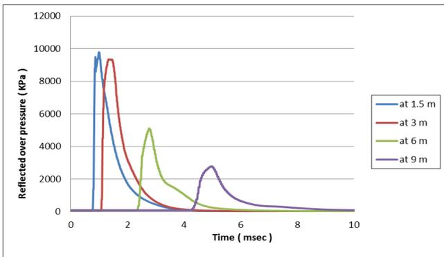
**Fig.5:** reflected overpressure histories at mid height of column C1 of building A - load case 1.
