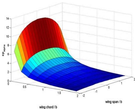
Fig 4. 3-D pressure distribution of rectangular wing (AR=2,  $k=0$ ,  $M=0$ ,  $N_x=10$ ,  $N_y=10$ ).
