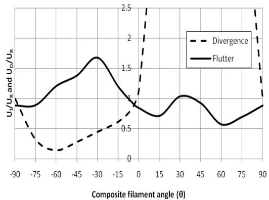
**Fig 19. Flutter and divergence speeds (U<sub>f</sub>, U<sub>D</sub>) normalized with respect to U<sub>R</sub>=44.67 m/s ( U<sub>D</sub> at θ=90°).**
