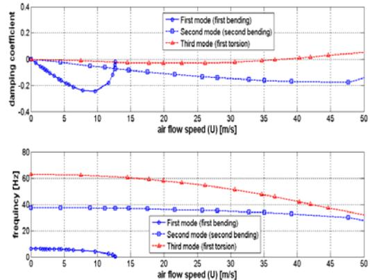
Fig 18. The U-g curve and U-frequency curve for a [-30/0]<sub>s</sub> plate wing.
