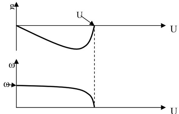
Fig 3. U-g and U- $\omega$  curves to find divergence speed ( $U_D$ ) [1].
