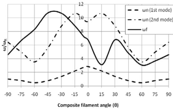
Fig 20. Flutter and natural frequencies ( $\omega_f, \omega_n$ ) normalized with respect to  $\omega_R=1.665$  rad/sec (1<sup>st</sup> natural frequency at  $\theta=90^\circ$ ).
