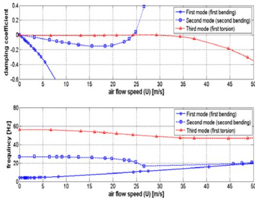
Fig 15. The U-g curve and U-frequency curve for a [+45/0]<sub>s</sub> plate wing.
