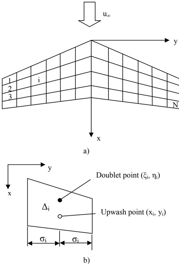
Fig 1. Aerodynamic elements in doublet point method [14].
