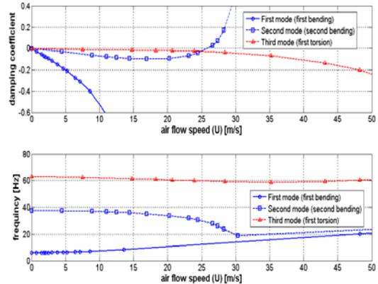
Fig 17. The U-g curve and U-frequency curve for a [+30/0]<sub>s</sub> plate wing.
