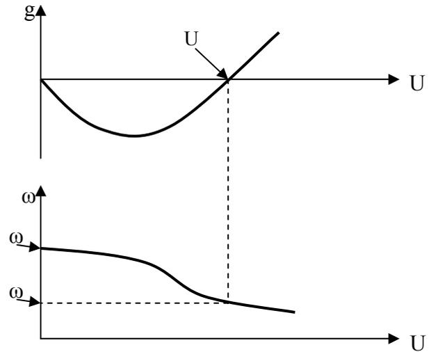
Fig 2. U-g and U- $\omega$  curves to find flutter speed and frequency ( $U_f, \omega_f$ ) [1].
