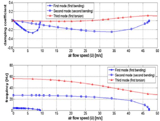
Fig 16. The U-g curve and U-frequency curve for a [-45/0]<sub>s</sub> plate wing.
