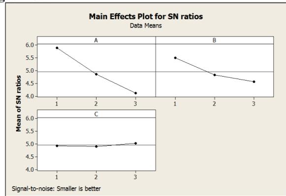
Fig.2: S/N ratio plot for surface roughness
