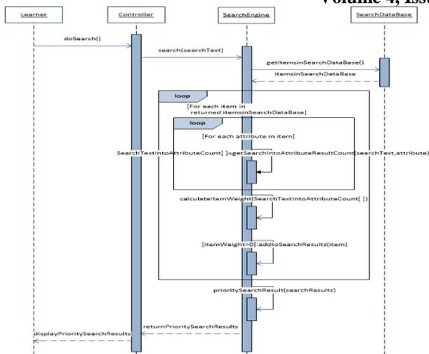
Fig. 8. UML sequence diagram for search engine
