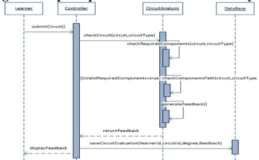
Fig. 6. UML sequence diagram for circuit analysis
