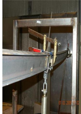
Photo 2. Warped beam
