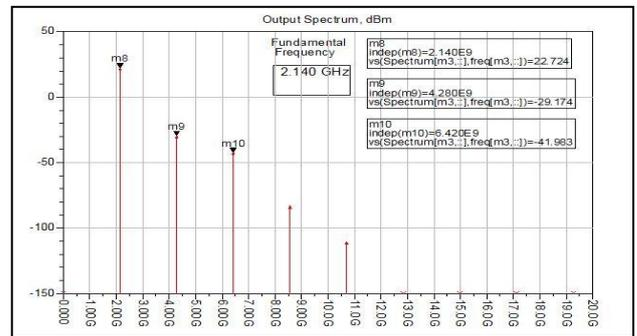
Fig (8): Output spectrum of the three-way DPA
