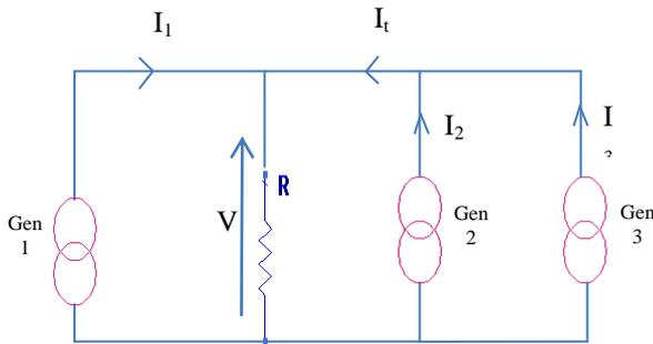
Fig (3): Active Load Pull schematic
