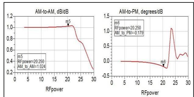
Fig (9): Amplitude distortion and Phase distortion
