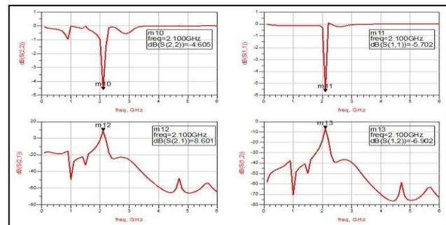
Fig (10): Results of the input and output matching of the three-way DPA design
