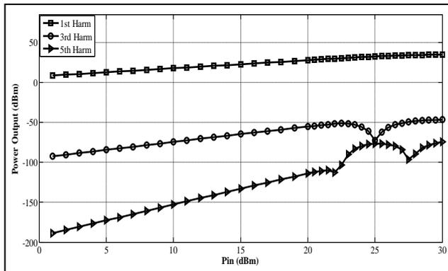
Fig (12): Power harmonics with input power
