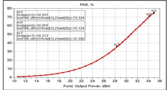
Fig (7): Power Added Efficiency (PAE%) of the 3-Way DPA design at  $P_{out,max}$ (m5), $P_{out,1dB}$ (m6) and  $P_{out,6dB}$  (m7)
