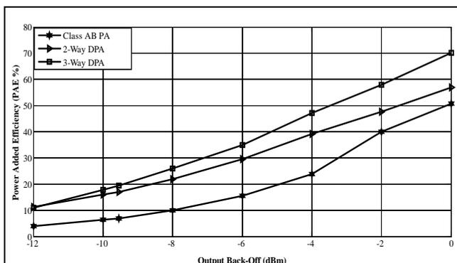
Fig (14): PAE of the conventional PAs and N-Way DPA with different output back-off points for W-CDMA base-station
