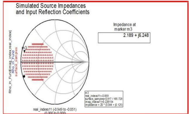
Fig (5): Source Pull Analysis to determine input impedance for maximum efficiency
