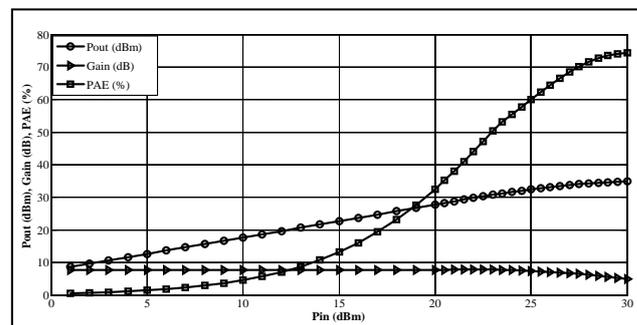
Fig (11): Output power, gain, and PAE as a function of input power
