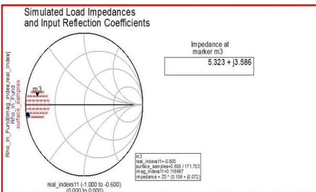
Fig (4): Load Pull Analysis to determine load impedance for maximum efficiency
