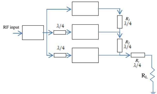
Fig (2): Block Diagram of three-way DPA
