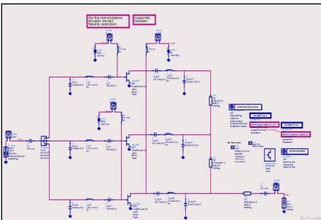
Fig (6): Schematic of the three-way Doherty power amplifier design
