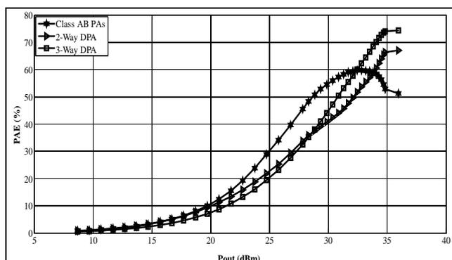
Fig (15): PAE of the conventional PAs and N-Way DPA with output power for W-CDMA base-station
