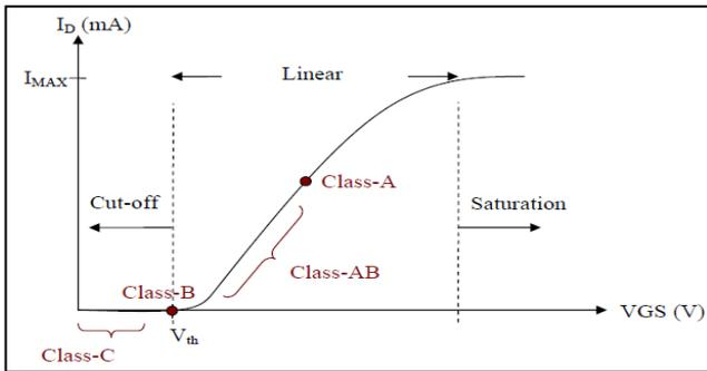
Fig (1): Classes of operation of Power amplifier based on transfer characteristics
