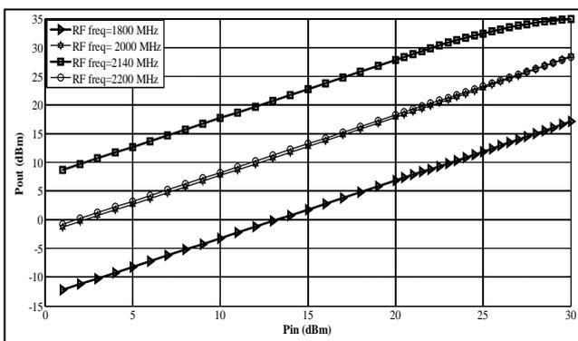
Fig (13): Output power as a function of input power for difference input signal frequencies
