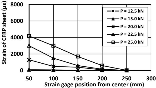
Fig. 16. Strain distribution of H-1-30 specimen.
