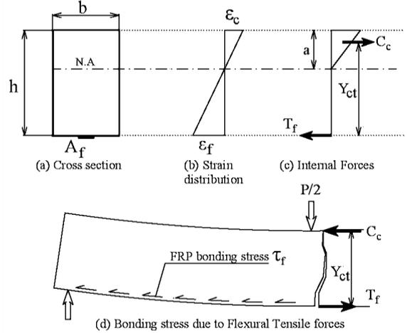
Fig. 10. Bonding stress in flexural beam.
