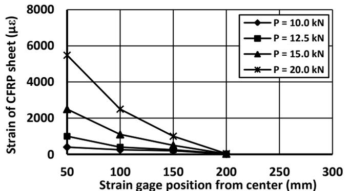
Fig. 15. Strain distribution of H-1-15 specimen.
