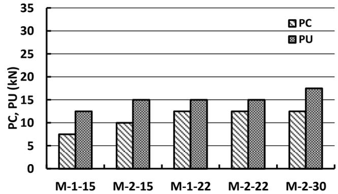
**Fig. 4 Effect of CFRP length and stiffness on cracking and ultimate loads (group II).**
