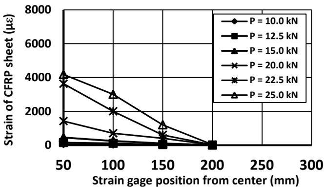
Fig. 18. Strain distribution of H''-1-15 specimen.
