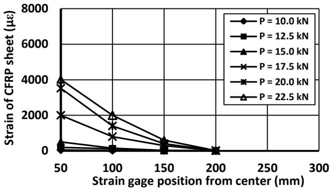
Fig. 17. Strain distribution of H'-1-15 specimen.
