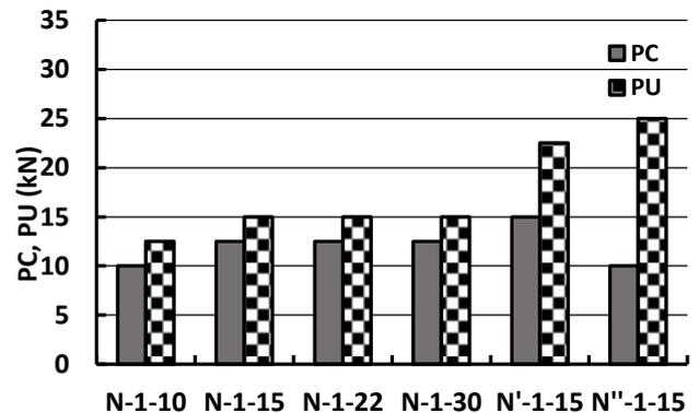
**Fig. 3 Effect of CFRP length, width, and roughness surface on cracking and ultimate loads (group I).**
