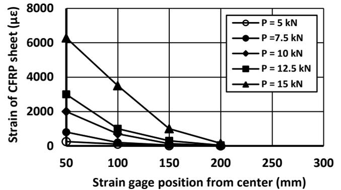
Fig. 12. Strain distribution of N-1-15 specimen.
