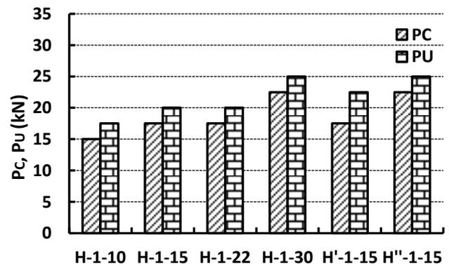
**Fig. 5 Effect of CFRP length, width, and roughness surface on cracking and ultimate loads (group III).**
