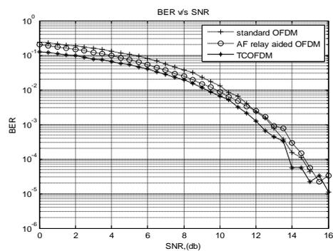
**Fig. 13. Comparison of BER curve of standard, AF relayed and TCOFDM**
