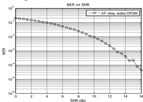
**Fig. 9. BER curve of AF relay aided OFDM**
