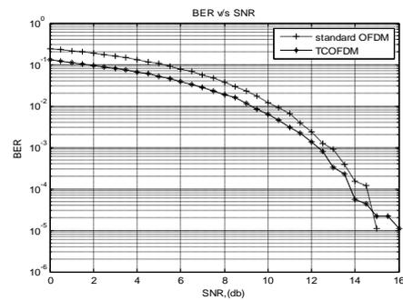
**Fig. 12. Comparison of BER curve of standard OFDM and TCOFDM**
