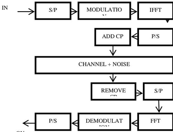
Fig. 1. Block diagram of OFDM
