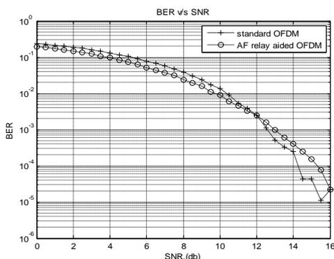
**Fig. 10. Comparison of BER curve of standard OFDM and AF relay aided OFDM**
