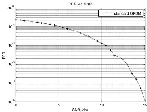
**Fig. 8. BER curve of standard OFDM**
