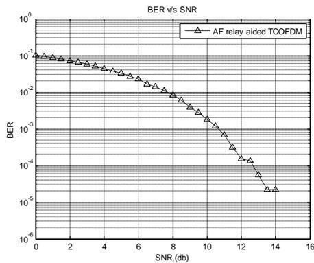
Fig. 14. BER curve of AF relay aided TCOFDM
