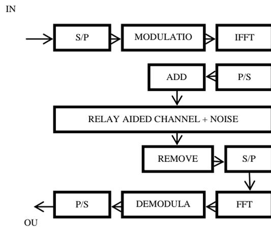
Fig. 3. Block diagram of relay aided OFDM
