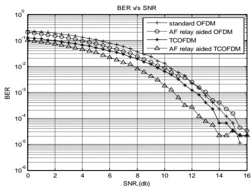
Fig. 15. Comparison of BER curve of standard, AF relayed, TCOFDM and AF relay aided TCOFDM
