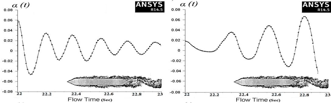
Fig.13 Time histories of torsional displacement for deck section (2).
