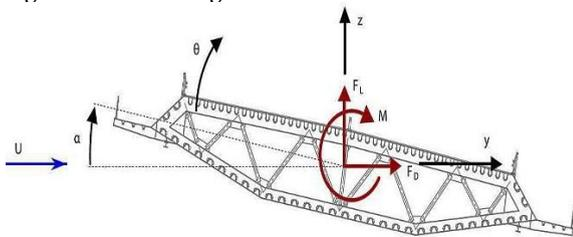
Fig. 3 Sign criteria for the aerodynamic Forces [4].
