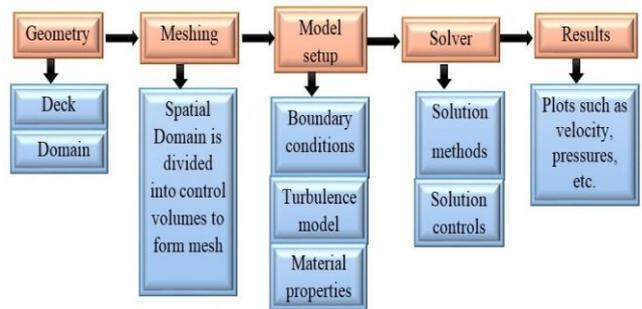
**Fig. 6 Flow chart for "CFD methodology" over bridge deck**
