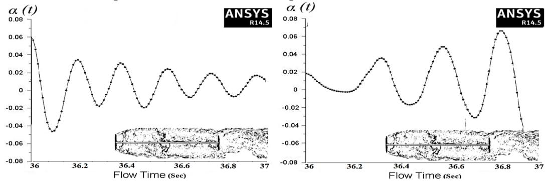
Fig.15 Time histories of torsional displacement for deck section (4).
