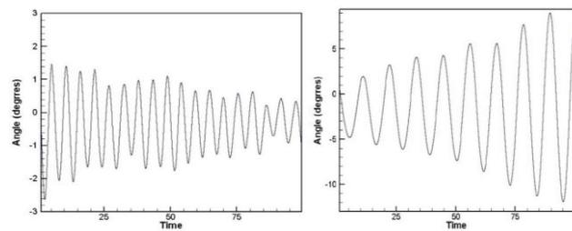
(a) Positive damping (b) Negative damping
