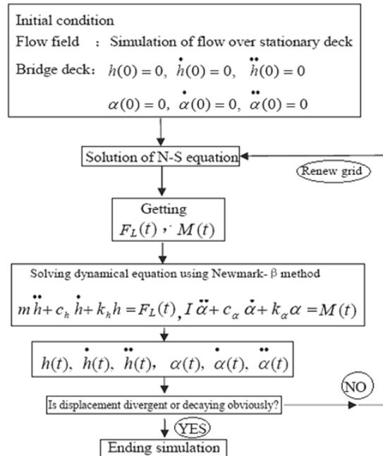
Fig. 4 Procedure of FSI in every wind speed [5]
