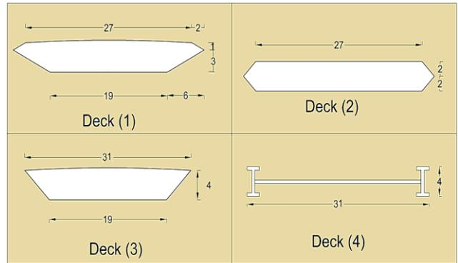
**Fig. 5 Geometric definition of the deck cross sections**
