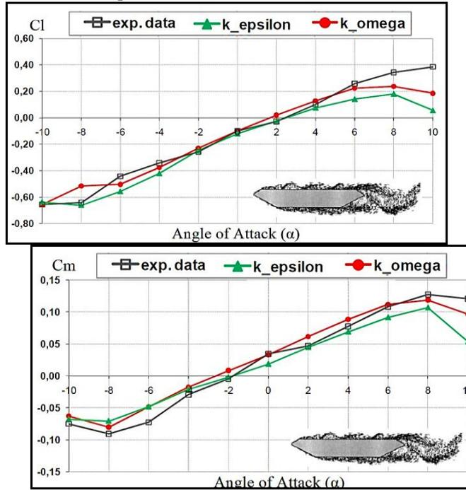
(a) Lift coefficient ( $C_l$ ) (b) Moment coefficient ( $C_m$ )
