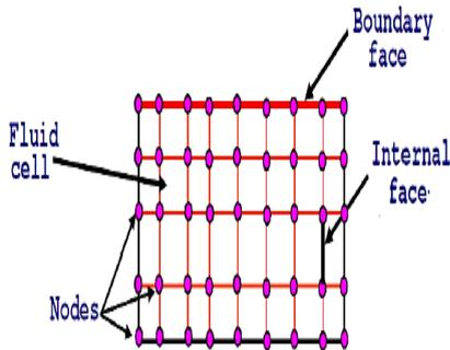
Fig. 8 Definition of cells, nodes, and face [7]
