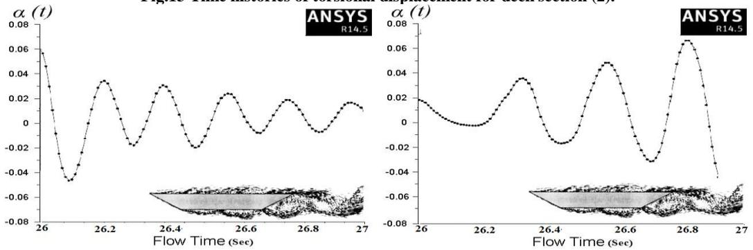
Fig.14 Time histories of torsional displacement for deck section (2).
