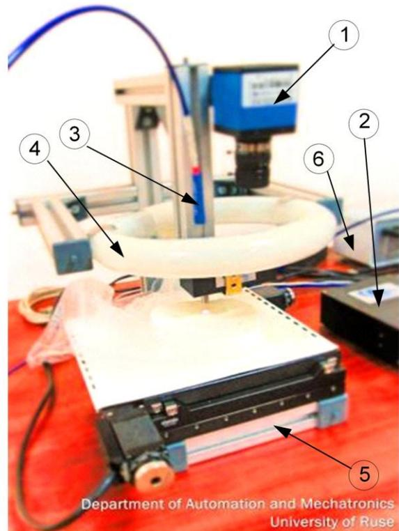
Fig. 9. Hyperspectral imaging system based on point scanning: 1 – RGB camera DFK 31AU03; 2 – QE65000 spectrophotometer; 3 – spectrophotometer probe; 4 – illumination system; 5 – SMTF-102LS05 XY motorized scanning stage; 6 – SSMC4-USBhF stage motion controller.
