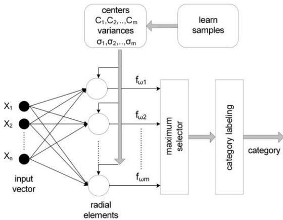
Fig. 7. Classifier architecture with spherical radial basis elements.
