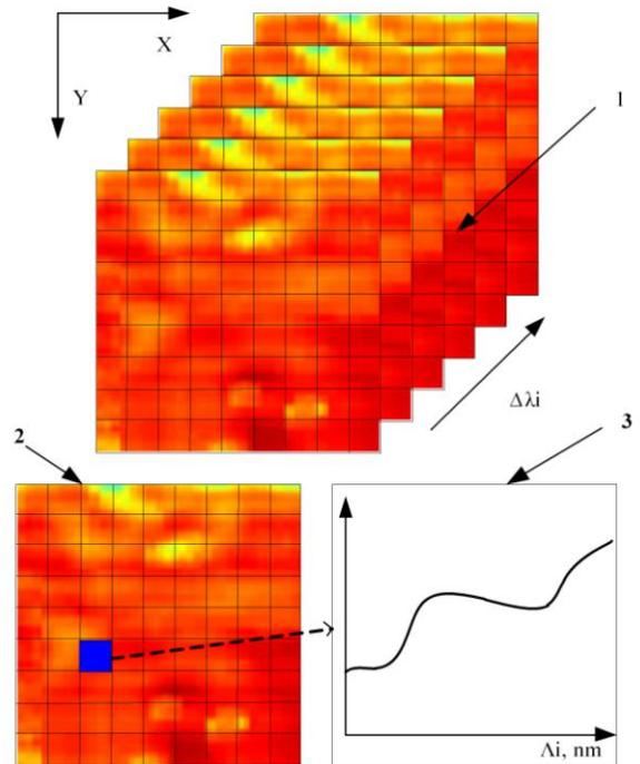
**Fig. 3. Schematic representation of the relation between spectral and spatial characteristics in hyperspectral imaging: 1 – set of images in different narrow bands  $\Delta\lambda_i$ ; 2 – plane image (X-Y) from one bandwidth  $\Delta\lambda_i$ ; 3 – spectral characteristic of one particular pixel from the plane image for  $\Delta\lambda_i$ .**
