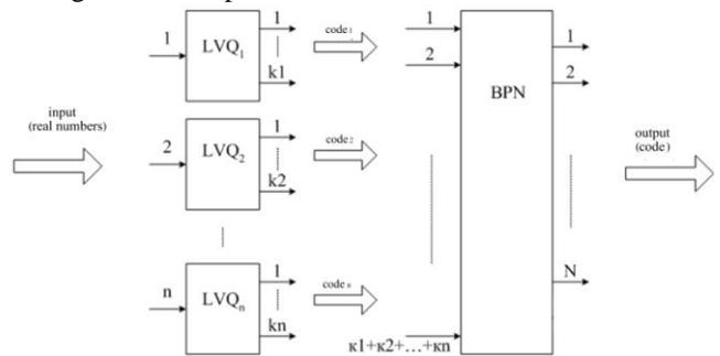
**Fig. 5. Network architecture, defining class areas of in the form of parallelepiped (CCNN)**
