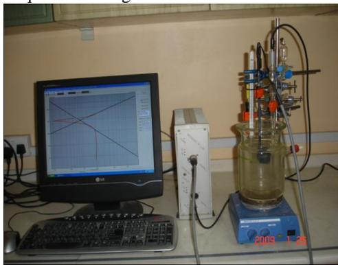
Fig (2) the electrochemical corrosion unit
