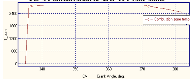
Fig. 5 Combustion zone temperature Vs Crank angle
