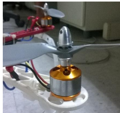
Fig. 8 Propeller driven by brushless DC motor being released to simulate the flight failure
