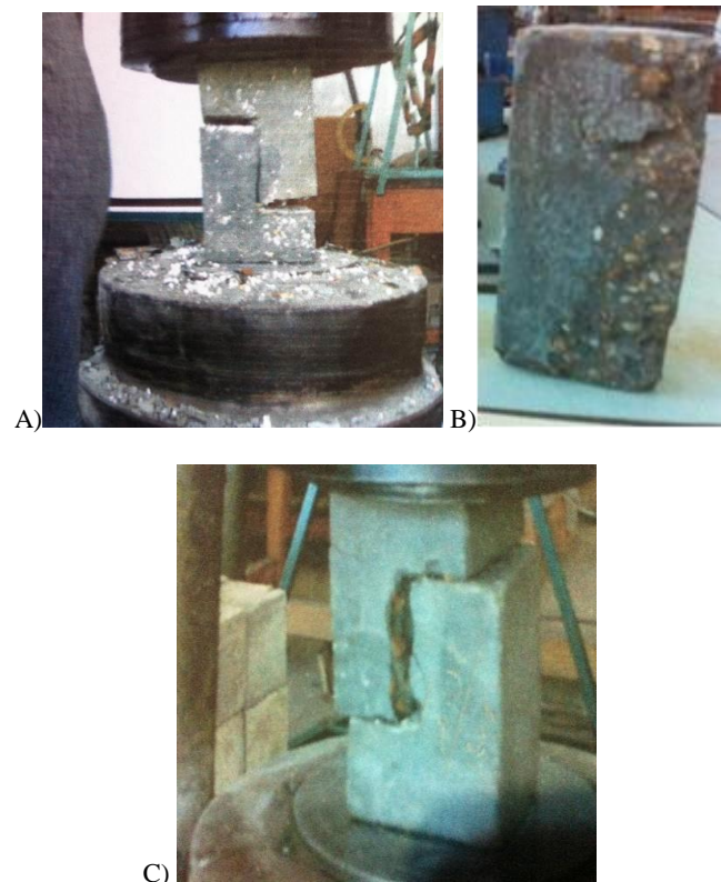
Fig. 6 Specimens after failure; A: Bond Failure, B: Mix Failure, C: Non-Bond Failure.
