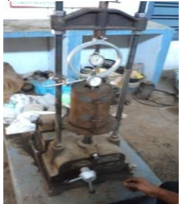
Fig: 1 California Bearing Ratio Test Apparatus
