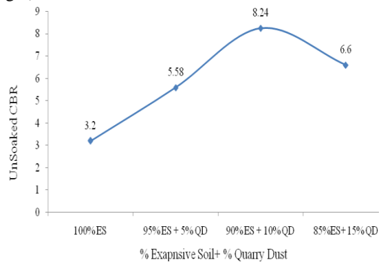
Fig.6 Variation Of Un Soaked CBR with Increase in % of Quarry Dust.
