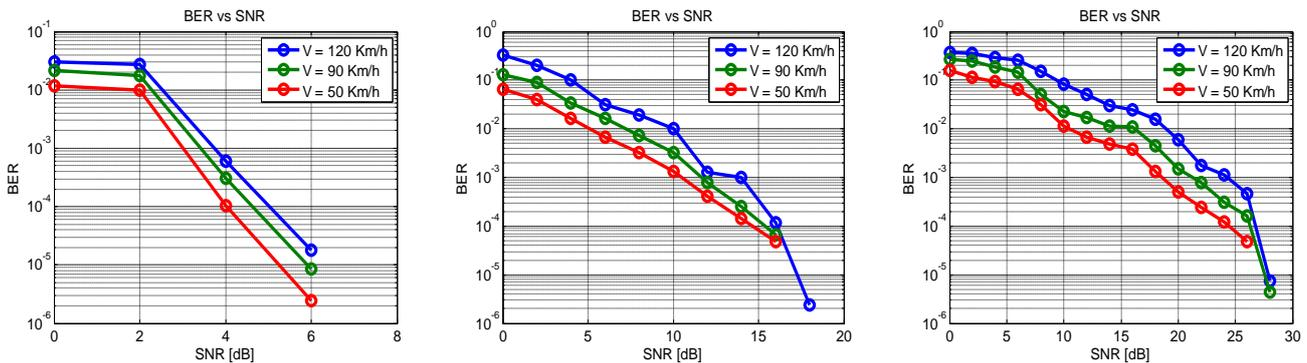
Fig. 11. BER vs SNR compared Mobile Velocities and Modulations (V2X Communication): a) QPSK, b) 16QAM, c) 64QAM
