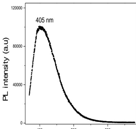
**Fig.2. Fluorescence spectra of Ce<sup>3+</sup> doped BLN glasses, λ<sub>ex</sub> = 350 nm**
