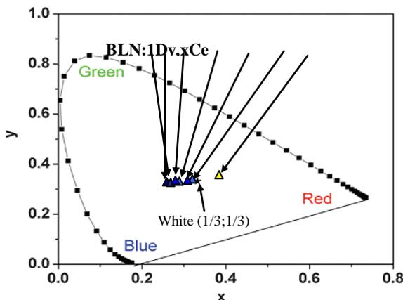
**Fig.5. CIE chromaticity diagram for 1%mol  $Dy^{3+}, xCe^{3+}$  co-doped in BLN glass**
