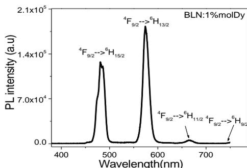
**Fig. 1. The emission spectrum of BNL: 1% Dy<sup>3+</sup> glass, λ<sub>ex</sub> = 386 nm.**
