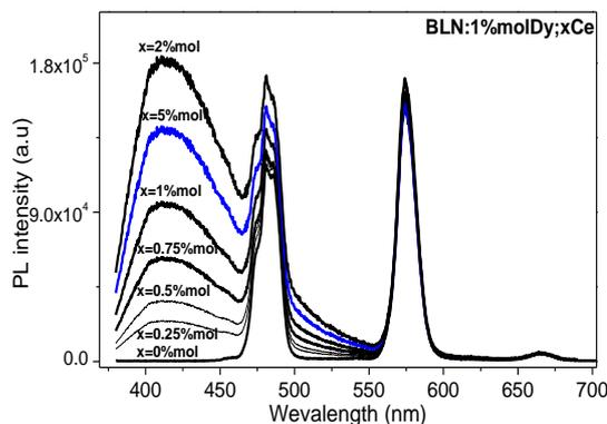
**Fig. 4. Fluorescence spectra of Dy<sup>3+</sup>, Ce<sup>3+</sup> co-doped in BNL glass, λ<sub>ex</sub> = 350 nm.**
