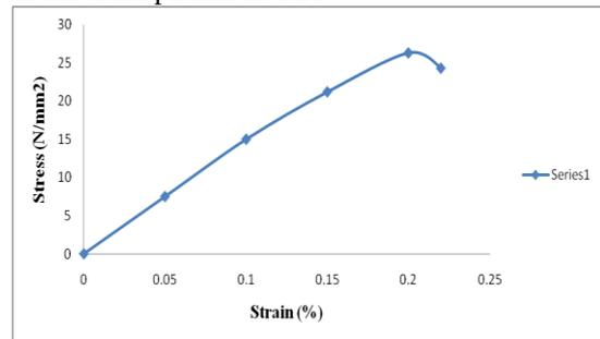
**Fig 1: Stress-strain response for concrete with 0% polypropylene fibre**
