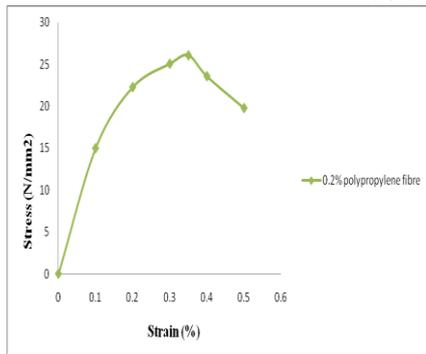
**Fig 3: Stress-strain response for concrete with 0.2% polypropylene fibre**
