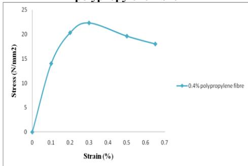
**Fig 5: Stress-strain response for concrete with 0.4% polypropylene fibre**
