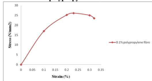
**Fig 2: Stress-strain response for concrete with 0.1% polypropylene fibre**
