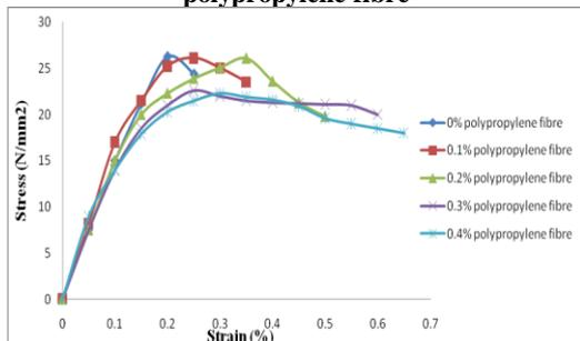
**Fig 6: Stress strain response of FBC at different volume fraction of polypropylene fibre**
