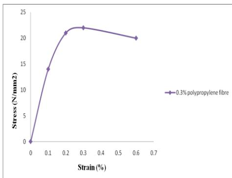
**Fig 4: Stress-strain response for concrete with 0.3% polypropylene fibre**
