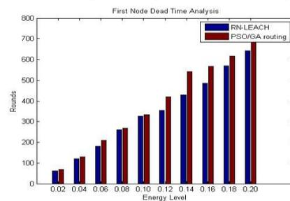
**Fig .1 Graph when first node dies in RN- LEACH and PSO/GA routing.**
