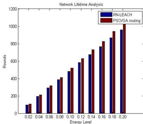
Fig 2 Graph for Network Lifetime in RN-LEACH and PSO/GA routing
