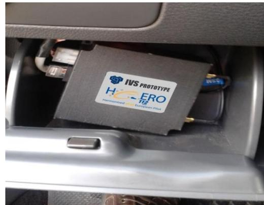
**Fig. 3 IVS+ device installed in the service compartment of a test car**
