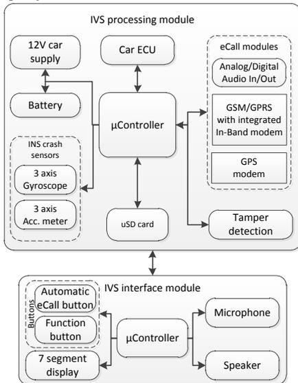
**Fig. 2 Structure of the device with additional functions**
