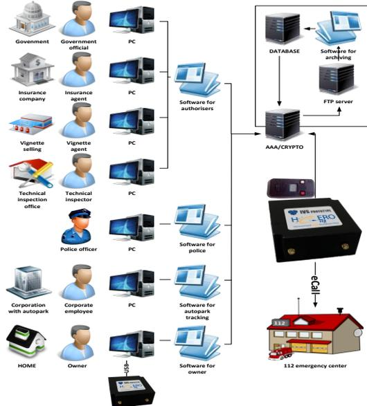
**Fig. 1 Block diagram of the system for car park management and accident signaling through eCall**
