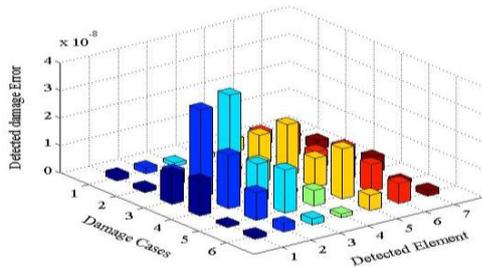
Fig (14) Damage Detection Error for double 50% Damaged elements.
