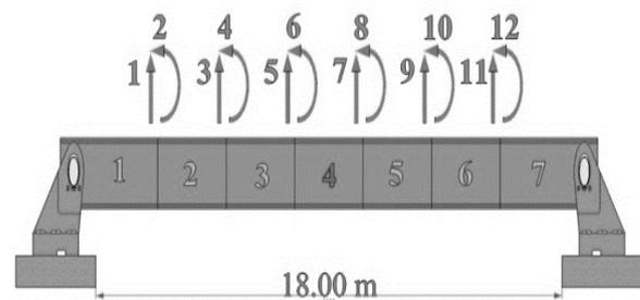
Fig (1) Simple Beam with All DOFs.
