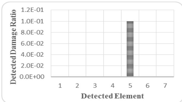
Fig (2): Detected Damage Ratio for 10% Damage in element number five.
