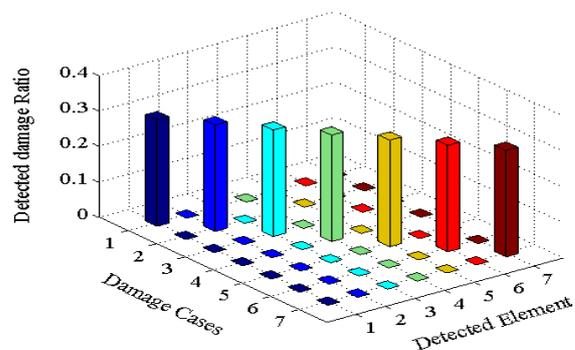
Fig (6) Detected Damage Ratio for Single 30% Damaged elements.
