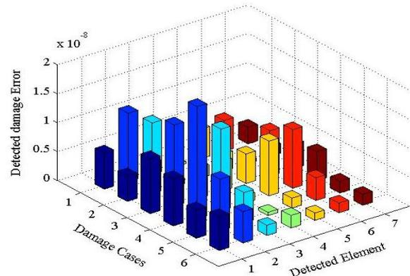
Fig (12) Damage Detection Error for double 10% Damaged elements.
