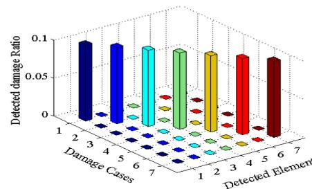
Fig (4) Detected Damage Ratio for Single 10% Damaged elements.
