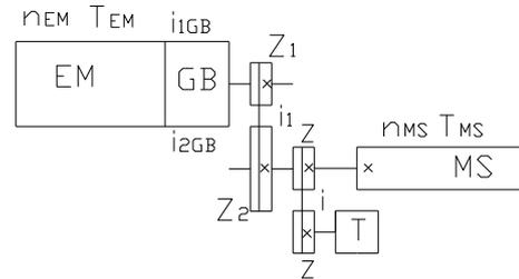
**Fig.4. Kinematic scheme of the main kinematic chain with direct link and torque amplification**
