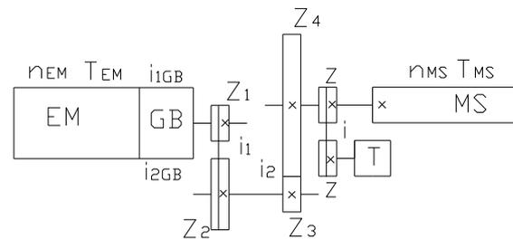
**Fig.5. Kinematic scheme of the main kinematic chain with direct link and two-stage reduction**
