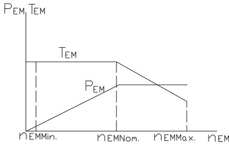
Fig.8. Electric motor characteristics
