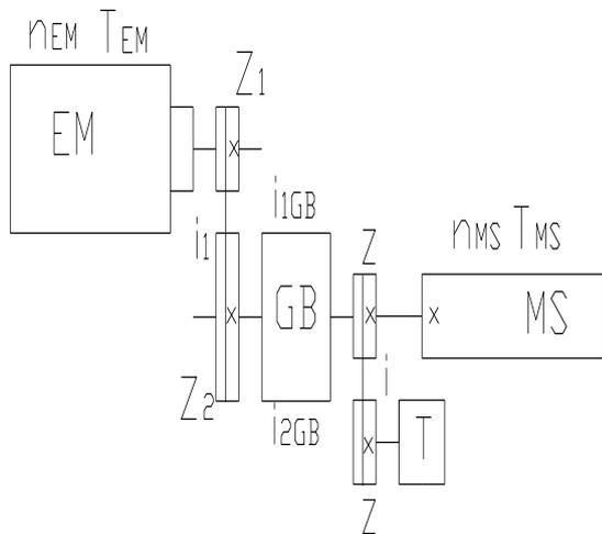
Fig.6. Kinematic scheme of the main kinematic chain with toothed belt transmission from electric motor to gear box
