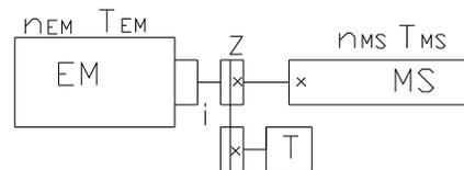
Fig.2. Kinematic scheme in the case of direct drive
