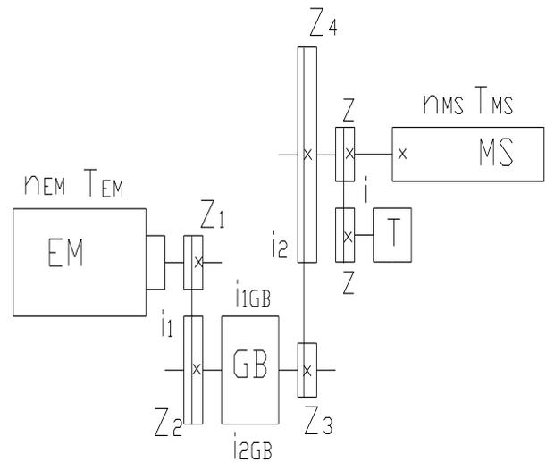
Fig.7. Kinematic scheme of the main kinematic chain with toothed belt transmission from electric motor to gear box and from this to main spindle
