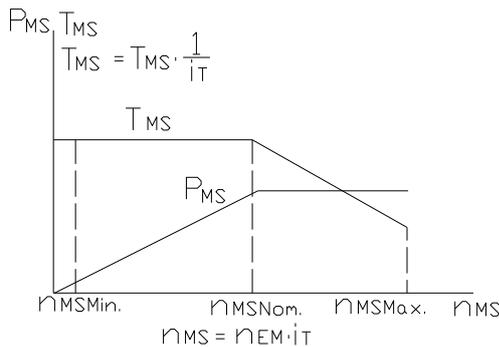
Fig.9. Torque/rotation and power/rotation characteristics of the main spindle
