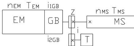
**Fig.3. Kinematic scheme of the main kinematic chain with direct link between electric motor and gear box**
