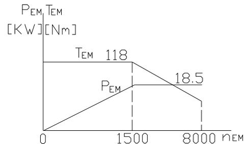
Fig.12. Characteristics of the new electric motor
