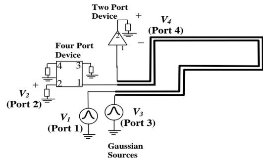
Fig 2. Coplanar four port and two port devices connected to adjacent signal traces
