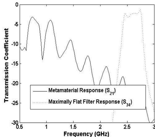
Fig. 9. The transmission response of a metamaterial coupler and a maximally flat filter when connected in a coplanar circuit environment to adjacent signal traces.
