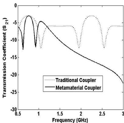
Fig. 7. The transmission response of the traditional and metamaterial couplers when the input is provided at port 1 and output is determined at port 2. The same response is observed at port 3.
