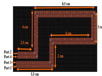
Fig 1. Schematic diagram of the two adjacent signal traces that are separated by a 100  $\mu$ m distance, as simulated in the Agilent Momentum.
