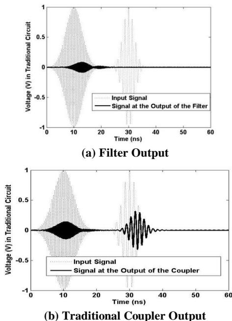
**Fig. 10. The 2.5 and 0.75 GHz Gaussian pulses as they appear at the output of (a) the traditional coupler and (b) the maximally flat filter centered at 0.75 GHz. at the filter's output, single deterioration is visible**
