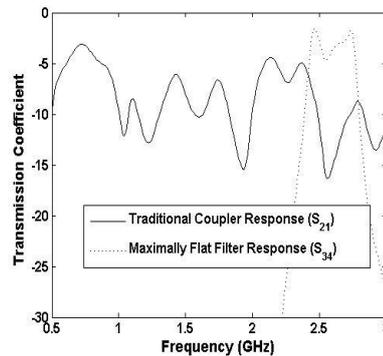
Fig. 8. The transmission response of a traditional coupler and a maximally flat filter when connected in a coplanar circuit environment to adjacent signal traces.
