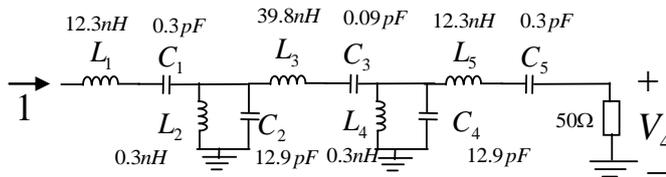
**Fig. 3. Schematic diagram of a Maximally-flat five stage band pass filter**
