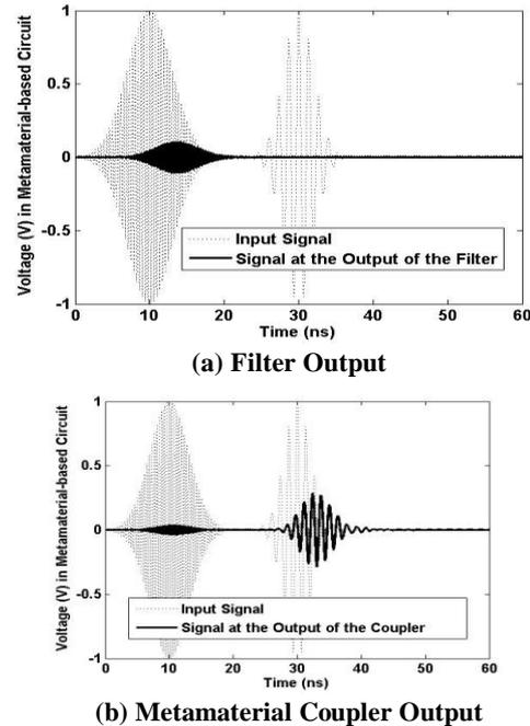
**Fig. 11. The 2.5 and 0.75 GHz Gaussian pulses as they appear at the output of (a) the metamaterial coupler and (b) the maximally flat filter centered at 0.75 GHz. The output pulse at the filter's output is much cleaner. The second harmonic at the output of the coupler is suppressed.**
