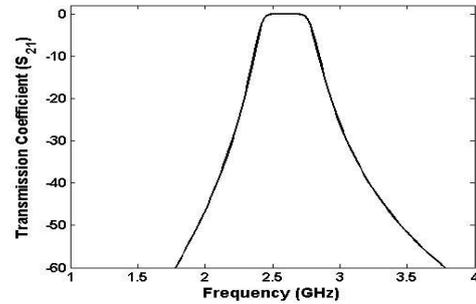
**Fig. 4. The transmission characteristics of the maximally flat bandpass filter centered at 2.5 GHz**
