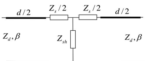
Fig. 6. The metamaterial unit cell used to implement the rate-race coupler. The design has been performed in [6]
