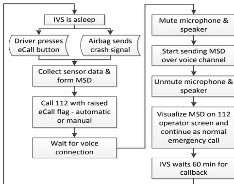
Fig. 2 Normal eCall workflow
