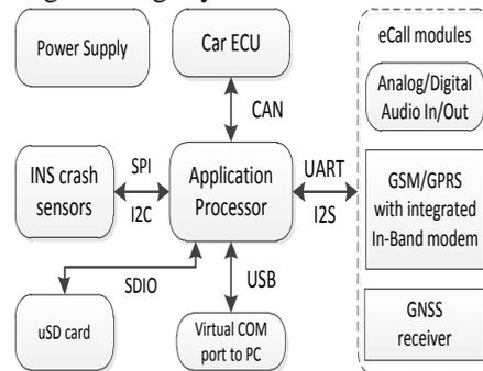
Fig.4 Structure of TUS’s IVS prototype
