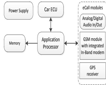
Fig.3 Basic structure of a real-life IVS device
