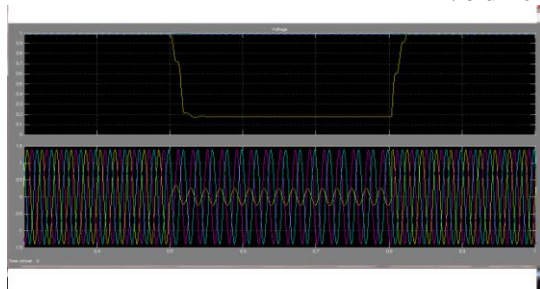
Fig.5 (a) : Voltage(rms) waveform & Fig.5 (b) :Phase to ground Voltage waveform of all the three phases R,Y & B
