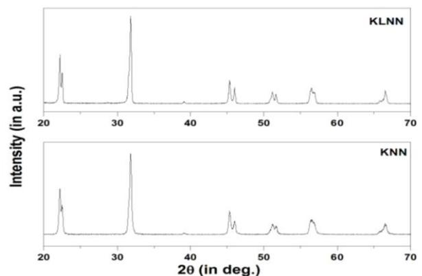
Fig 1. X-ray Diffraction patterns of calcined KNN and KLNN samples.
