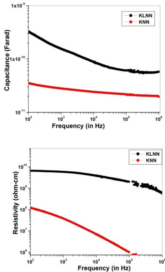
**Fig 3. Variation in capacitance and resistivity with frequencies up to 1 MHz at room temperature for KNN and KLNN samples.**
