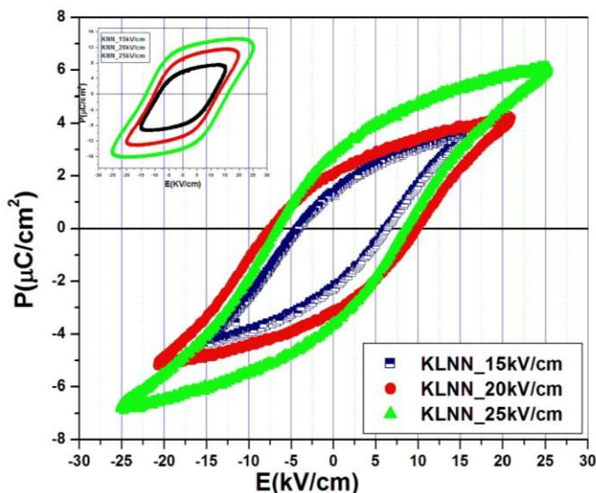
Fig 4. Ferroelectric behavior of KNN and KLNN at different applied electric fields.
