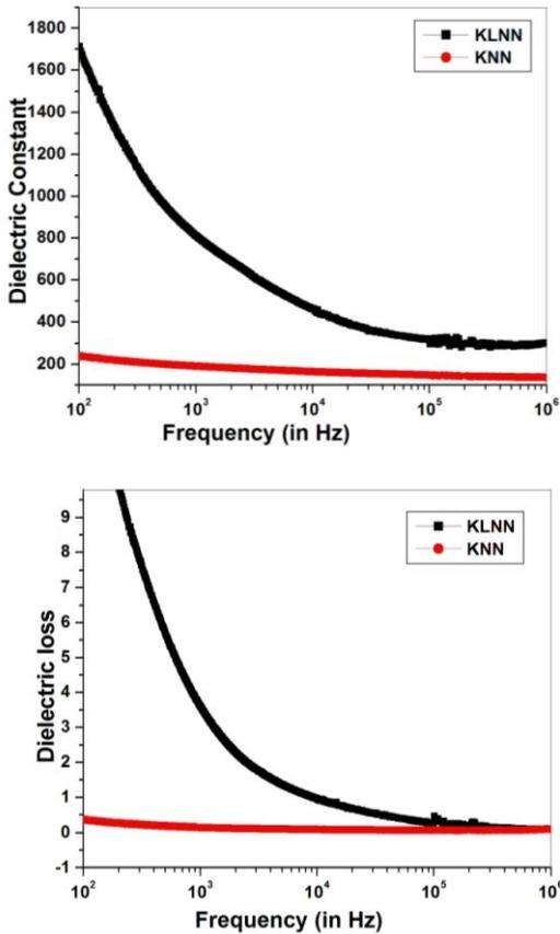
**Fig 2. Variation in dielectric constant and dielectric loss with frequency at room temperature for KNN and KLNN.**
