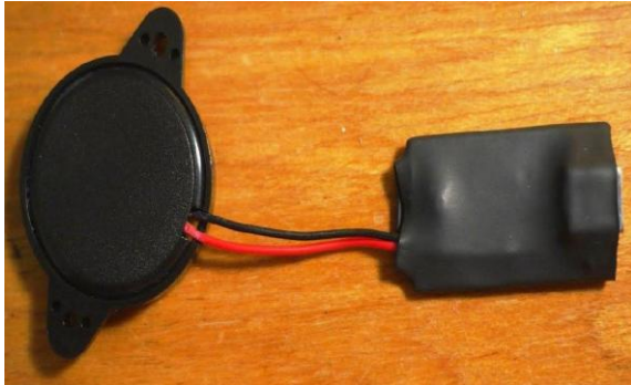
Fig (1): Simple low decibel transducer-Strokes from 0.10"
