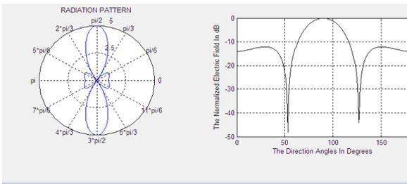
**Fig 2: Beam pattern without optimization 5 elements**
