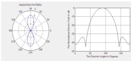
**Fig 3: Beam pattern with optimization 5 elements**
