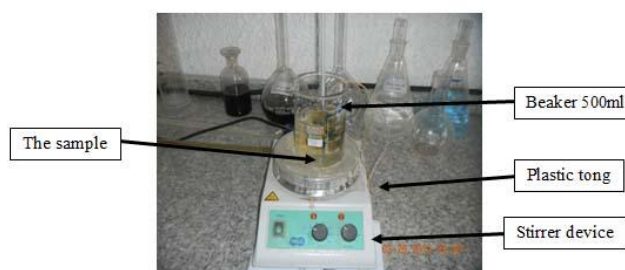
FIG. (2) CHEMICAL MACHINING SYSTEM
