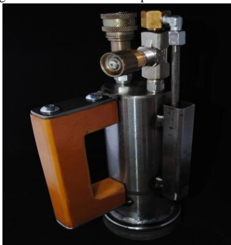
Fig 1. A Photograph of the Isolation Device Used by Global to Sample Hot Heat Transfer Fluids.
