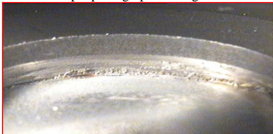
Fig. 13 Chamfer mark on gear with 6X magnification
