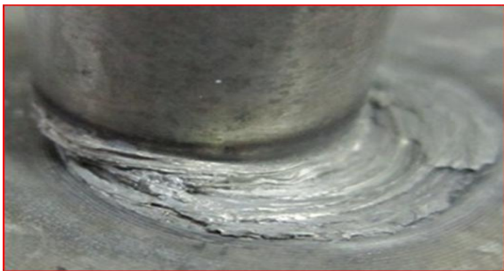
Fig. 6 Twist of shaft.
