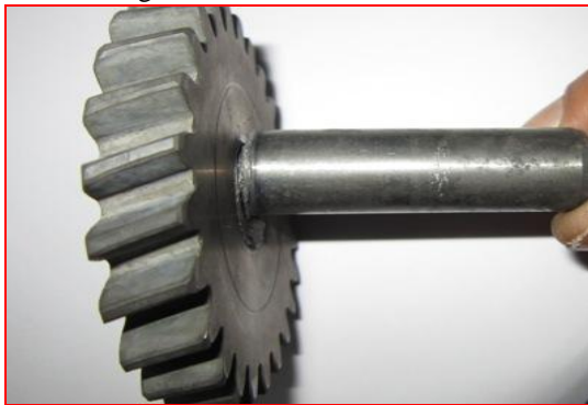
Fig. No. 12 Shaft bend near gear face.
