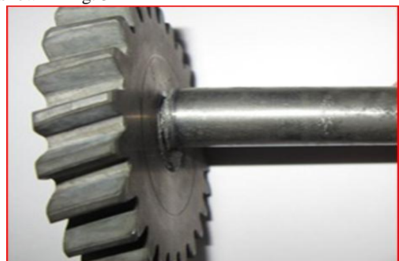
Fig. 3 Gear bend and shaft dislocate
