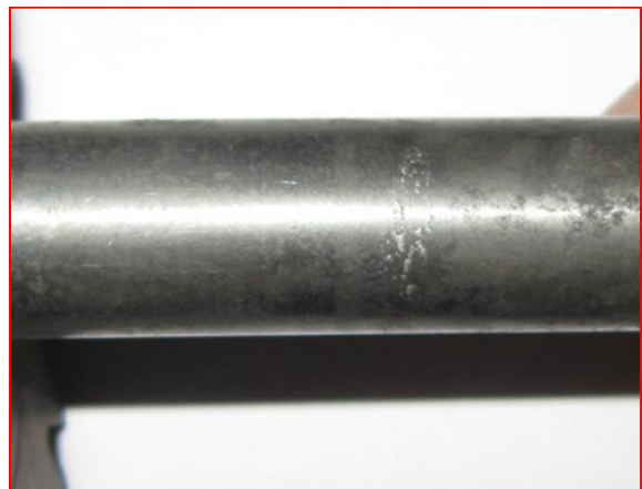
Fig. 10 Material deposited on the shaft.
