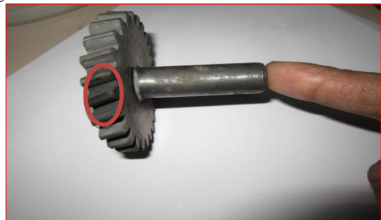
Fig. 1 Twisted shaft and gear assembly
