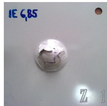
Fig.3 Sample sheet steel (90x90mm) with a basic coating (KTL)
