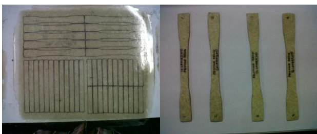
Fig. 4: GFRP Sheet and Tensile Test Specimen
