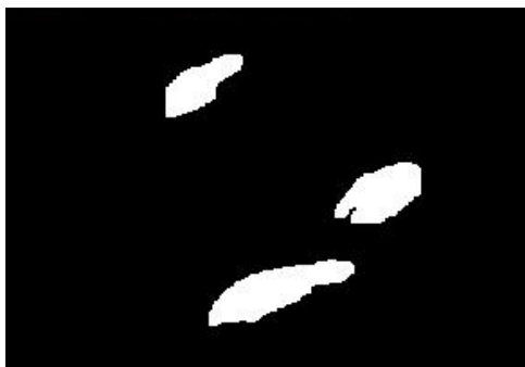
Fig.12: Dilation using disk of radius 3 as structuring element
