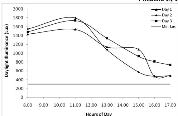
Fig-4: Daylight illuminance inside the Staircase at different hours of the day
