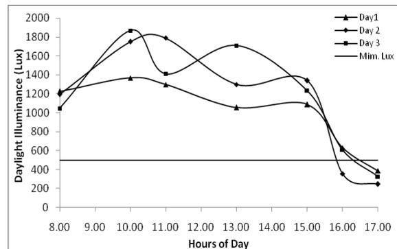
Fig-3: Daylight luminance inside the Foundry shed at different hours of the day
