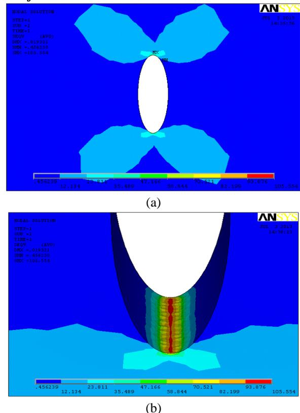
Fig.3. (a) and (b). Stress distribution around elliptical hole for  $b/a=0.2$
