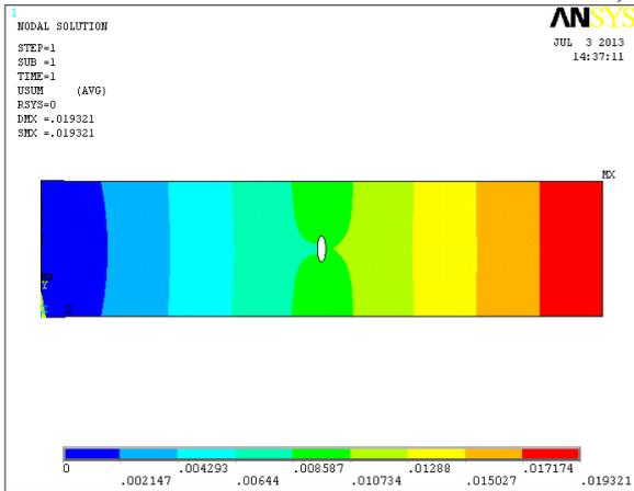
**Fig.4. Displacement due to the elliptical hole of aspect ratio (b/a) = 0.2**
