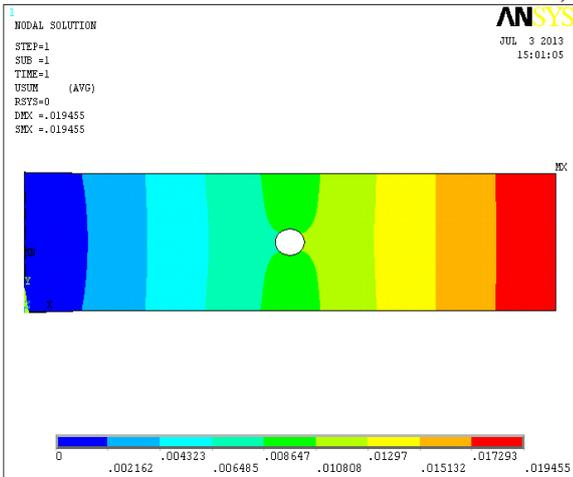
**Fig.12. Displacement due to the elliptical hole of aspect ratio (b/a) = 1.0**
