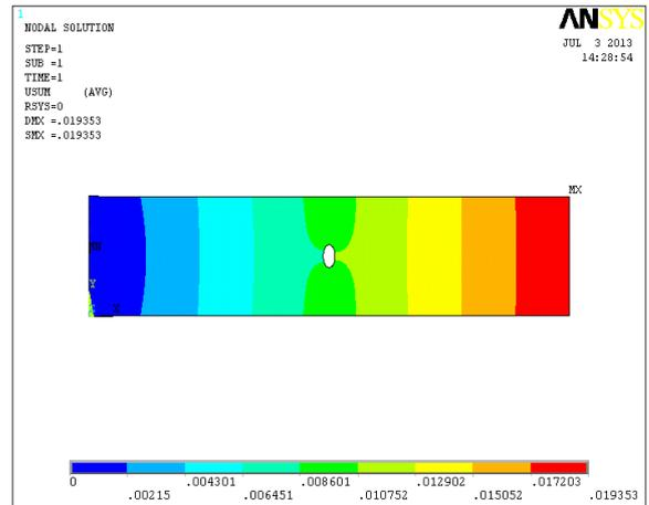
**Fig.6. Displacement due to the elliptical hole of aspect ratio (b/a) = 0.4**
