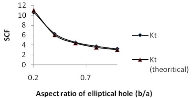
**Fig.15. Comparison between the theoretical SCF and value of SCF calculated using ANSYS**
