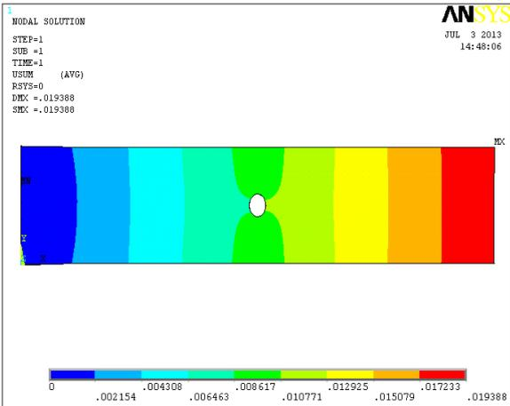
Fig. 8. Displacement due to the elliptical hole of aspect ratio (b/a) = 0.6
