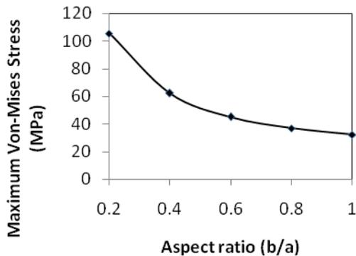
**Fig.13. Effect of aspect ratio of elliptical hole on the maximum stress**
