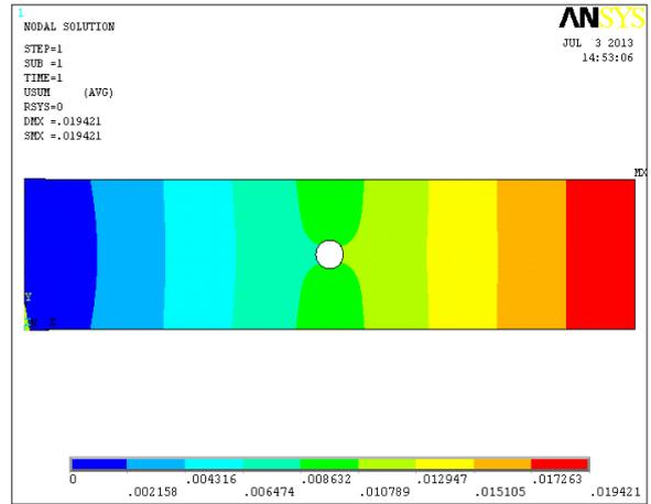
Fig.10. Displacement due to the elliptical hole of aspect ratio (b/a) = 0.8
