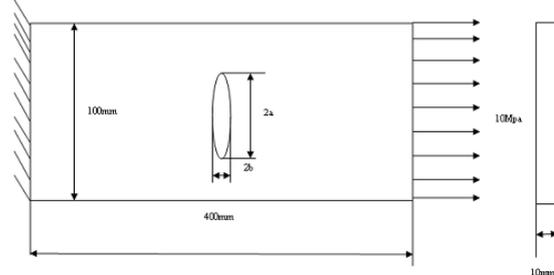
Fig.2. Geometry and boundary conditions of elastic plate with central elliptical hole
