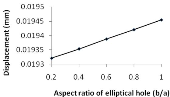
**Fig.14. Effect of aspect ratio of elliptical hole on the maximum displacement**
