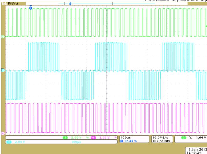
Fig.8. Unipolar PWM signals
