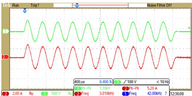
Fig.10. Output voltage and current waveform of power amplifier with feedback for 225Ω load
