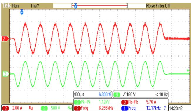
Fig.9. Output voltage and current waveform of power amplifier without feedback for 225Ω load.
