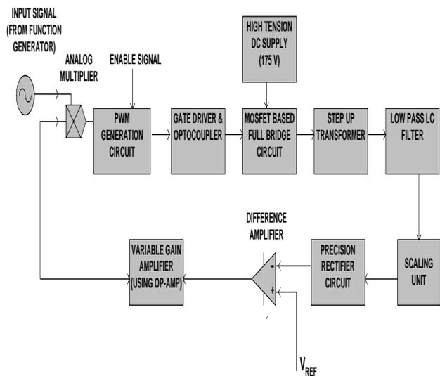
Fig.7. Power amplifier with analog feedback controller
