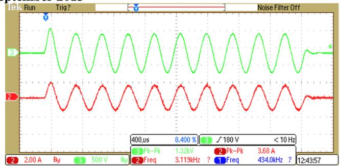
Fig 12. Output voltage and current waveform of power amplifier with feedback for 250Ω load
