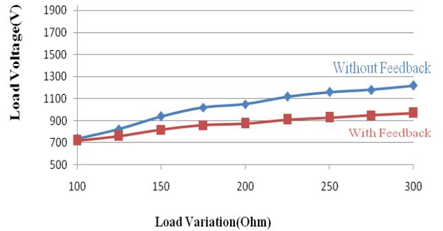
Fig 19. Load Vs output voltage
