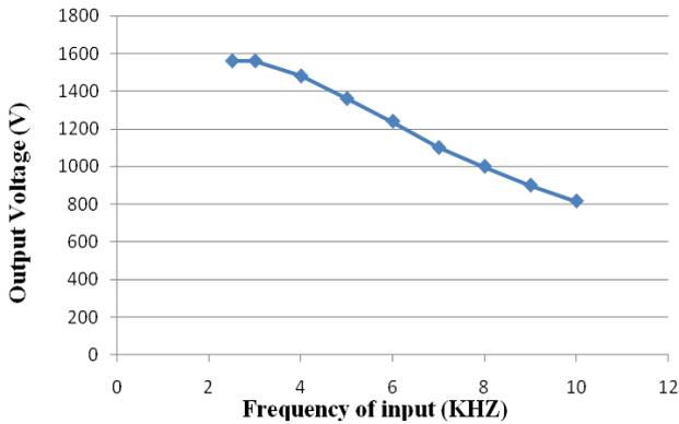
Fig 16. Frequency of Input Vs Output voltage
