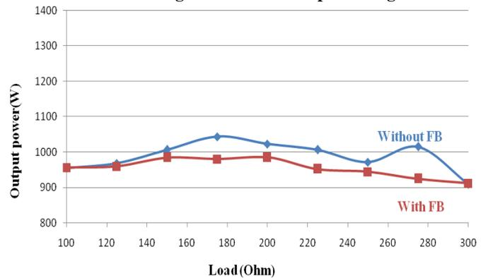
Fig 20. Load Vs output power
