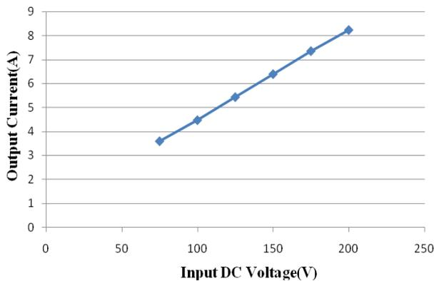
Fig 17. Input dc voltage Vs Output current
