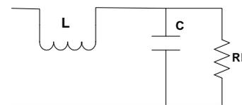
**Fig.6. 4<sup>th</sup> order low pass filter**
