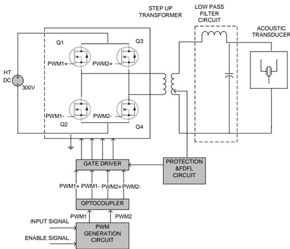
**Fig.4. Block diagram of Digital Power Amplifier without feedback system**
