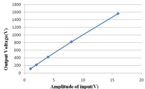
Fig 14. Amplitude of Input Vs Output voltage
