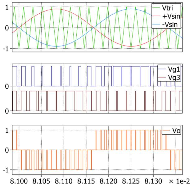
**Fig.2. Unipolar PWM signals**
