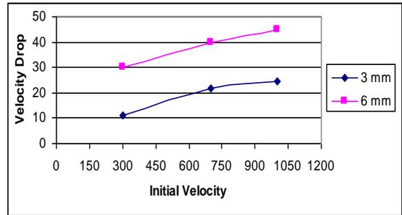
Fig.10 Comparison of velocity drop for 3mm and 6mm thickness plates
