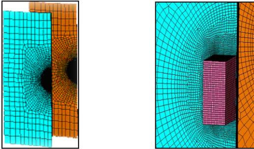
Fig.1 Discretization of geometry model
