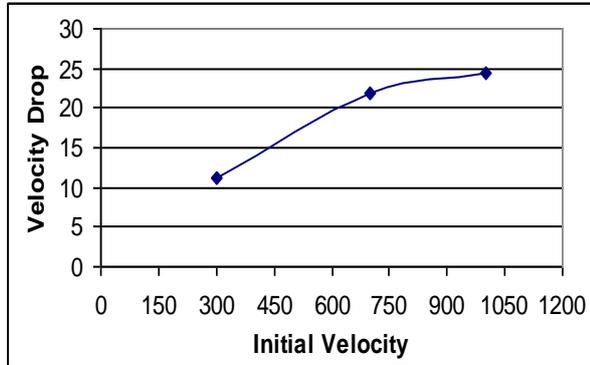
Fig.6 Velocity drop for Titanium and Aluminium plates (3mm)
