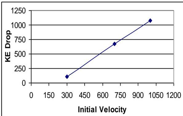
Fig.7 KE drop for Titanium and Aluminium plates (3mm)
