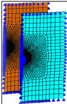
**Fig.4 Finite element model with boundary conditions**
