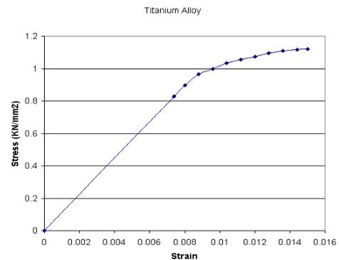
Fig.3 Stress-Strain curve for Ti alloy
