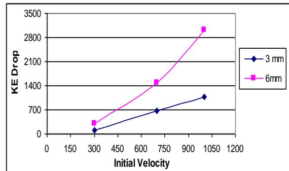
Fig.11 Comparison of KE drop for 3mm and 6mm thickness plates
