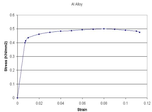
Fig.2 Stress-Strain curve for Al alloy
