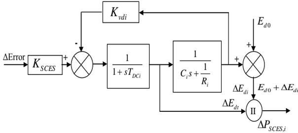
**Fig.2. Block diagram with capacitor voltage deviation feedback.**
