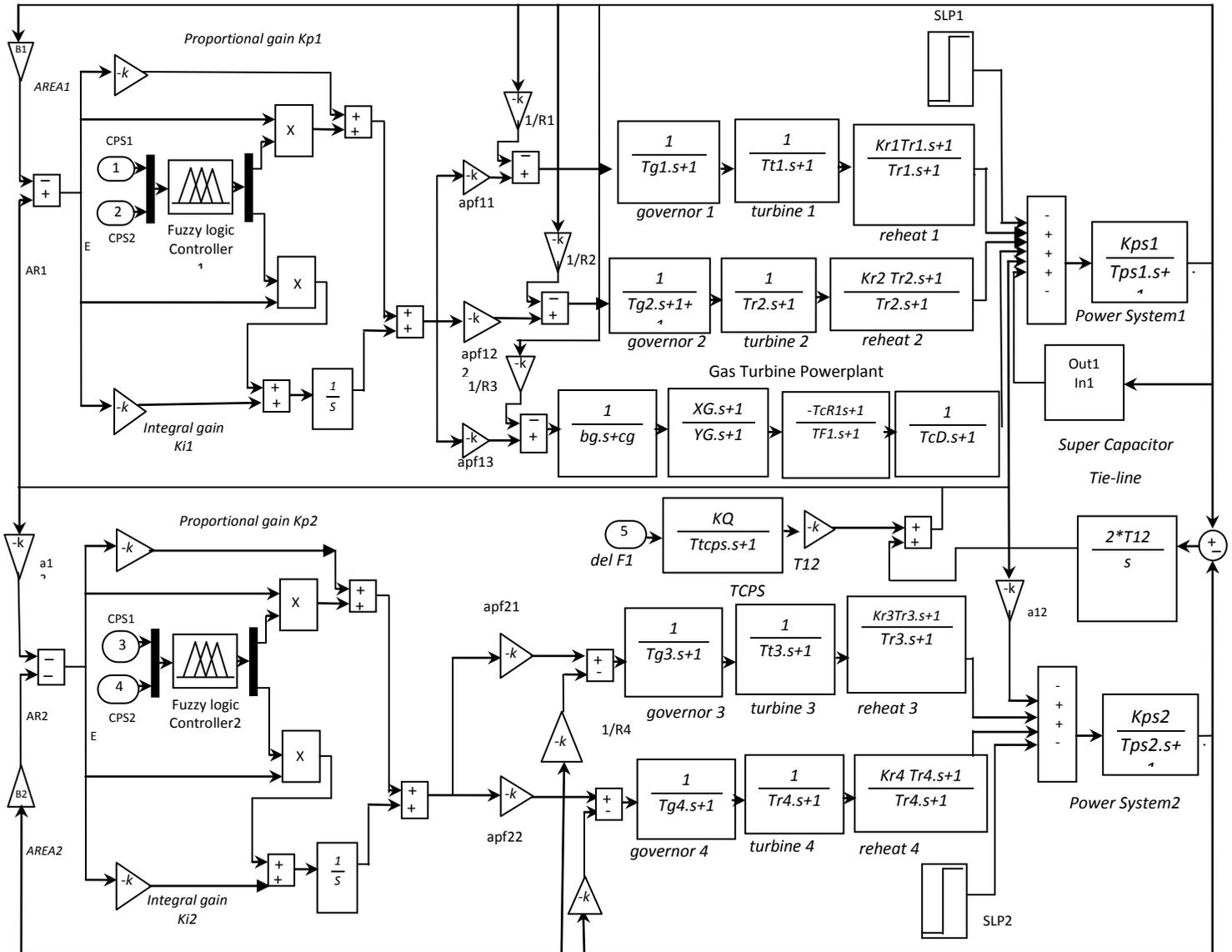
Fig. 8. Transfer function model of a two-area interconnected thermal reheat power system with TCPS and SCES units
