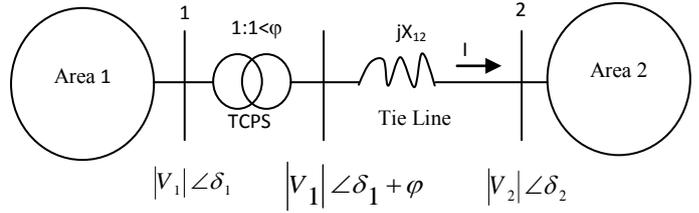
**Fig 3. A schematic of two-area reheat thermal power system with TCPS in Series with tie-line**
