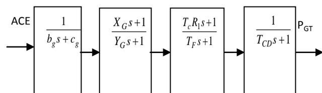
Fig. 1. Transfer Function representation of a Gas Turbine unit
