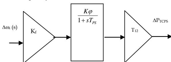
Fig 4. Structure of TCPS as a frequency Controller
